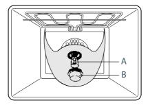
Fig.41 Removing either oven lamp
